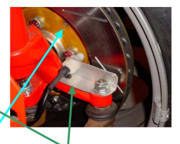
Magnets glued in position. Liberal application of a strong adhesive such as 'Chemical Metal' or 'Araldite' will ensure that the magnets do not become dislodged during use. Strong mounting brackets that hold the speed sensors in position. The brackets have been mounted in positions that move in unison with the magnets.
